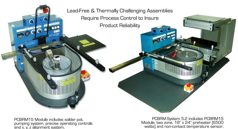
PCBRM15 Module includes solder pot, pumping system, precise operating controls and x, y, z álignment system.
